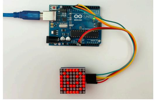
MAX7219 Display Module Interfacing with Arduino
