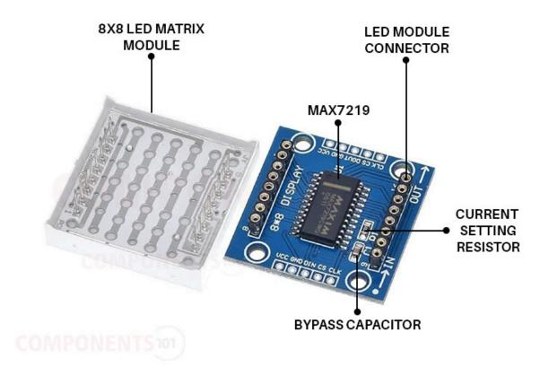
MAX7219 Display Module Parts Marking
