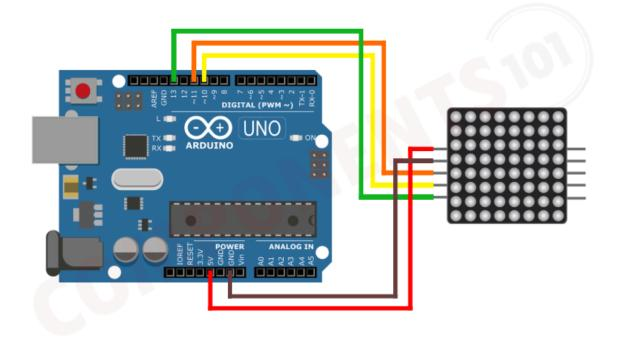
MAX7219 Display Module Interfacing Connection Diagram
