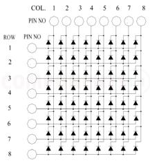
8x8 Dot-matix LED module Internal Circuit Diagram
