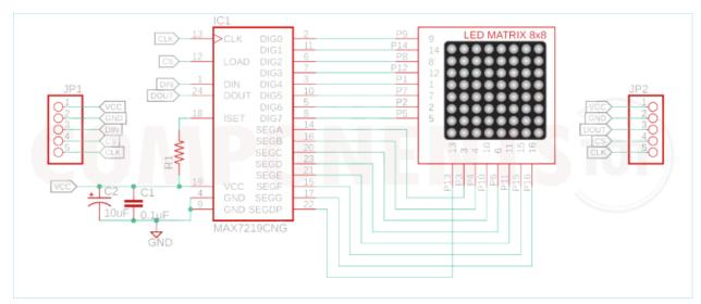
MAX7219 Display Module Circuit Diagram
