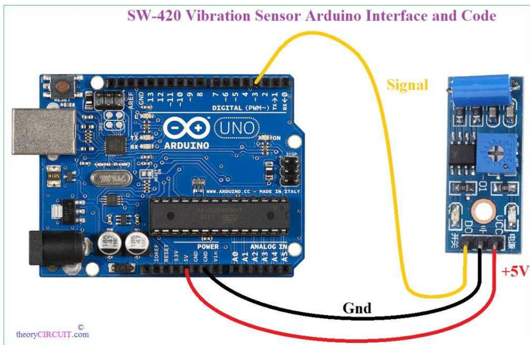
Connect Vcc pin of sensor board to 5V pin of Arduino board, connect Gnd pin to Gnd pin of Arduino, Connect DO output signal pin of sensor board to Arduino digital pin D3. Do some calibration and adjust the sensitivity threshold, then upload the following sketch to Arduino board.
