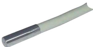
Sensors TF101U2 are encapsulated in a stainless-steel-shell V4A. They are suitable for measuring temperatures in fluids, under isolations, at surfaces or for inside or outside applications. The protection class is IP 66.
