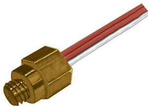
Platinum resistance temperature sensor on ceramic substrate built into a M6 brass threaded bush, especially suitable for being screwed into metal, e.g. for monitoring temperature of heat sinks or heating plates. Please note that there will be a measuring error due to the design, as the sensor can lose heat via the connection strand.
