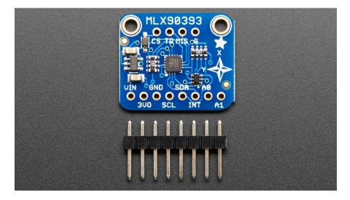
Measure the invisible magnetic fields that surround us, with this wide-range magnetometer. The MLX90393 is a wide range magnetic field sensor, that can measure 16-bits in ranges from +/-5mT up to +/-50mT in all 3 axes.
