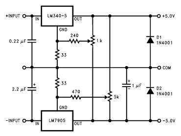
Figure 9. Dual Trimmed Supply
