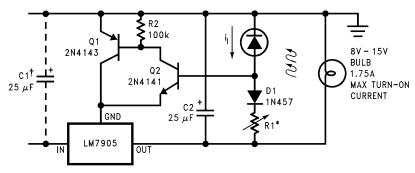
\*Lamp brightness increases until  $i_i$  = 5V/R1 ( $I_i$  can be set as low as 1  $\mu$ A) †Necessary only if raw supply filter capacitor is more that 2" from LM7905
