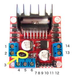
Connect the A+, A-, B+ and B- wires from the stepper motor to the module connections 1, 2, 13 and 14 respectively. Place the jumpers included with the L298N module over the pairs at module points 7 and 12. Then connect the power supply as required to points 4 (positive) and 5 (negative/GND).
