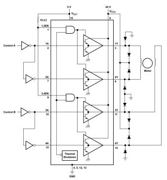
Figure 6. Two-Phase Motor Driver (L293)
