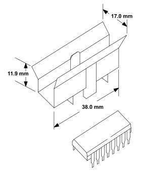
Figure 12. External Heat Sink Mounting Example ( $\theta_{JA} = 25^{\circ}$ C/W)
