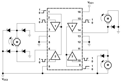
Output diodes are internal in L293D.
