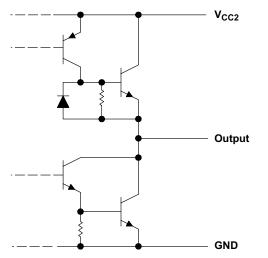
Figure 4. Schematic of Outputs for the L293
