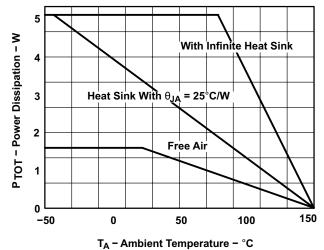
Figure 1. Maximum Power Dissipation vs Ambient Temperature
