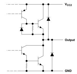
Figure 5. Schematic of Outputs for the L293D
