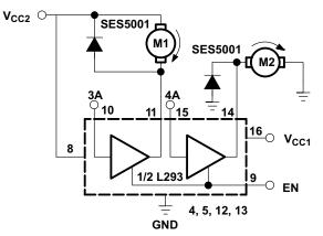
Connections to ground and to supply voltage
