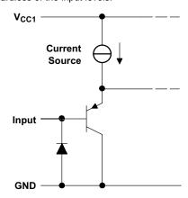
Figure 3. Schematic of Inputs for the L293x
