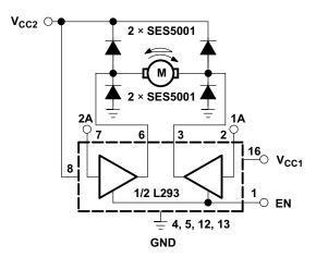
Figure 10. Bidirectional DC Motor Control
