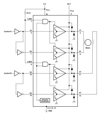
Figure 8. Two-Phase Motor Driver (L293D)
