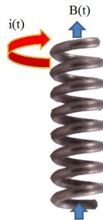
Fig. 1. A magnetic field is induced perpendicular to the direction of current flow through a coil of wire.
