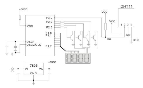
Connecting the typical application circuit shown above the microprocessor and DHT11, DATA pull-up and microprocessor I/O port.
