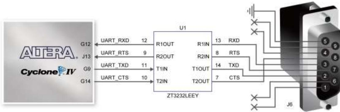
Figure 4-24 Connections between FPGA and ZT3232 (RS-232) chip
