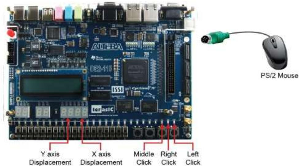
Figure 6-17 The setup of the PS/2 Mouse demonstration
