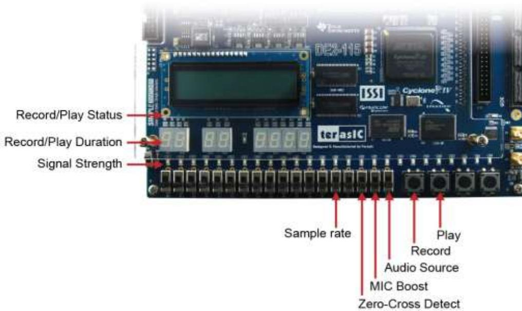
**Figure 6-25 Man-Machine Interface of Audio Recorder and Player**
