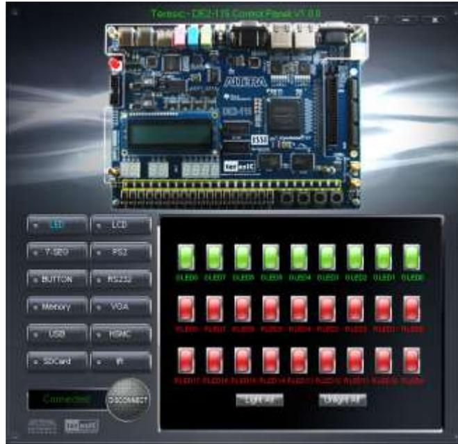
**Figure 3-3 Controlling LEDs**
