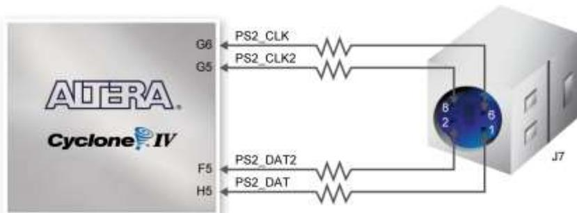
Figure 4-25 Connection between FPGA and PS/2
