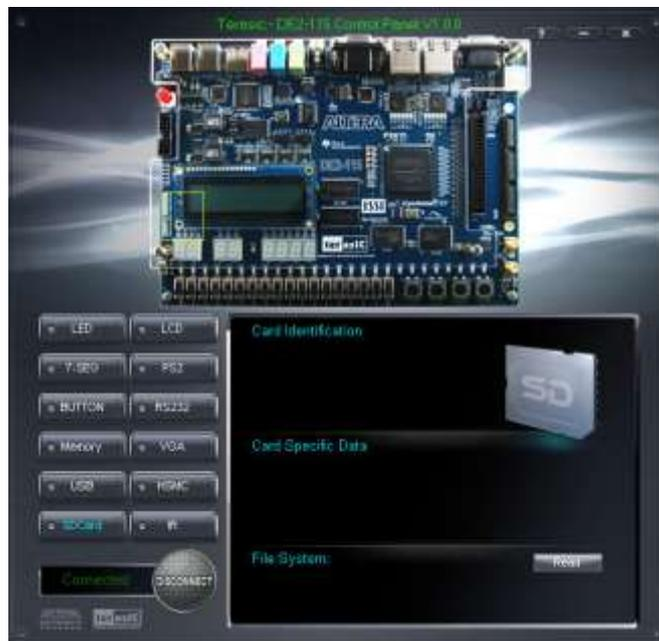
Figure 3-10 Reading the SD Card Identification and Specification
