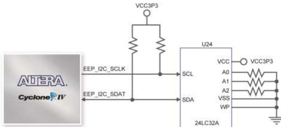
**Figure 4-36 Connections between FPGA and EEPROM**
