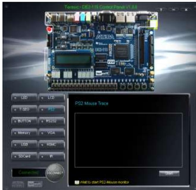
**Figure 3-9 PS/2 Mouse Monitoring Tool**
