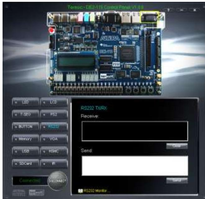
Figure 3-11 RS-232 Serial Communication
