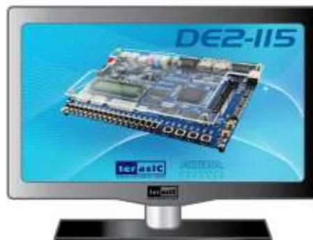
Figure 2-4 The default VGA output pattern
