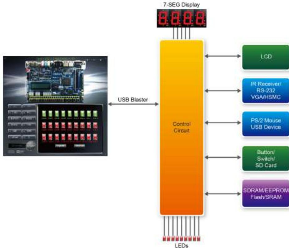
**Figure 3-2 The DE2-115 Control Panel concept**
