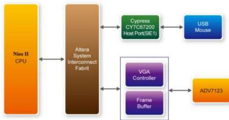
**Figure 6-3 Block diagram of the USB paintbrush demonstration**
