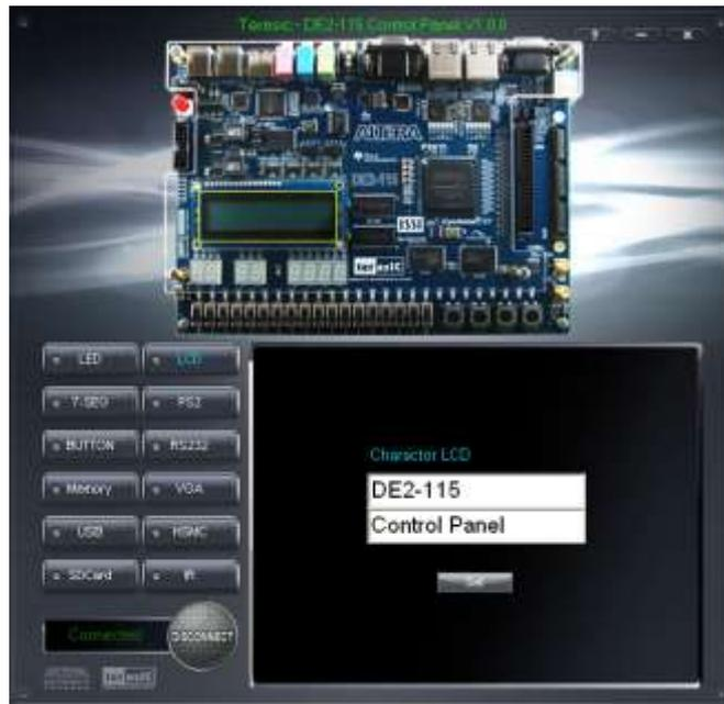
**Figure 3-5 Controlling the LCD display**
