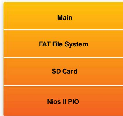
Figure 6-10 Software Stack of the SD Card Demonstration
