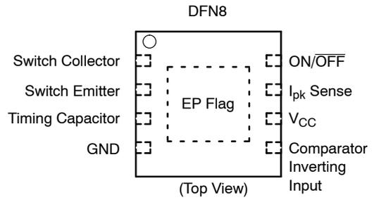
Figure 3. Pin Connections
