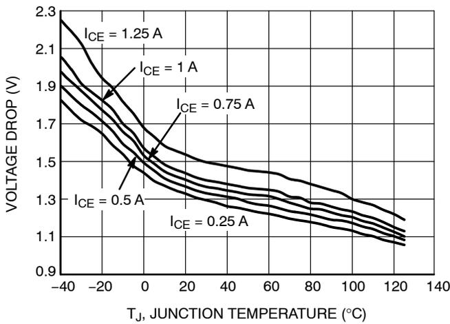
**Figure 7. Voltage Drop in Emitter Follower Configuration**
