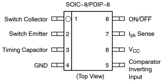
Figure 2. Pin Connections
