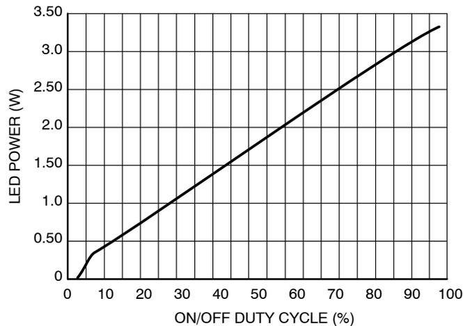
**Figure 26. Dimming Characteristic**
