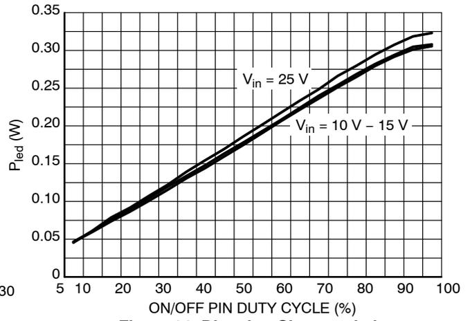
Figure 21. Dimming Characteristic
