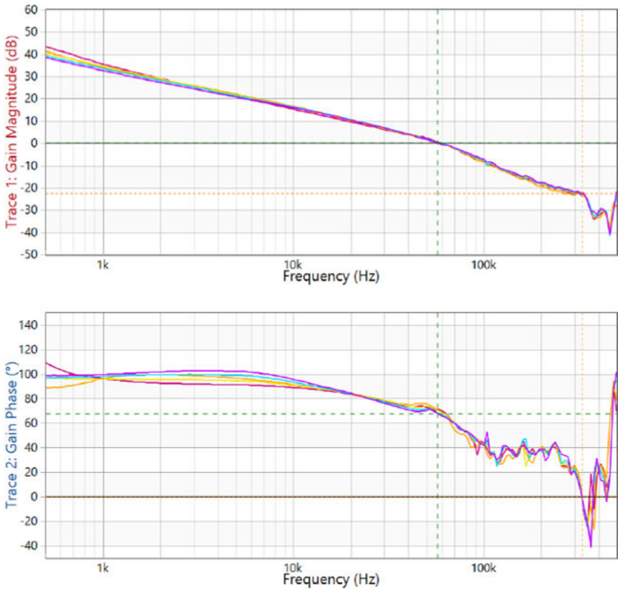
Figure 5-17. Stability Measurement: (Phase/Gain) Margin = 68 deg/22.5 dB, Cross-Over = 57 KHz
