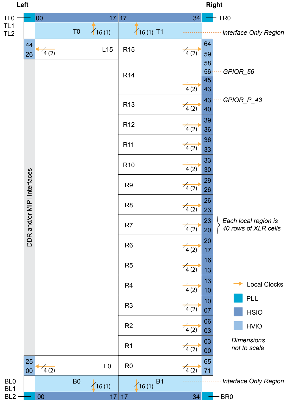
Figure 14: Clock Sources that Drive the Interfaces
