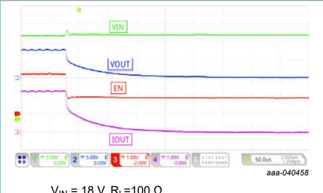
Fig. 19. Over temperature shutdown due to persistent input over voltage
