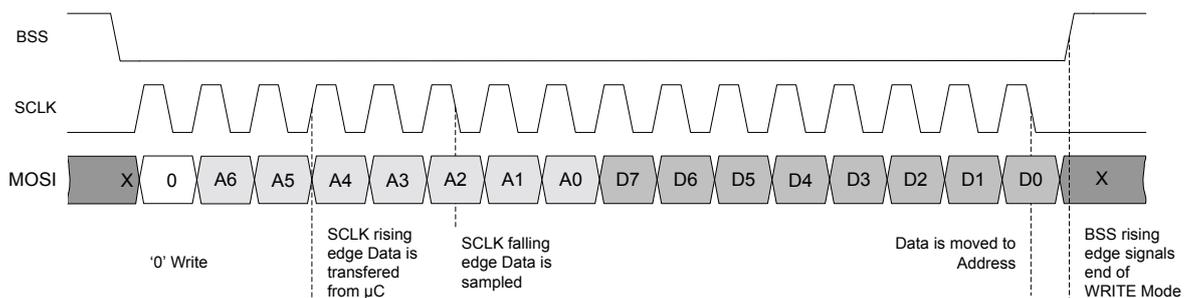
Figure 10. SPI communication: writing of multiple bytes
