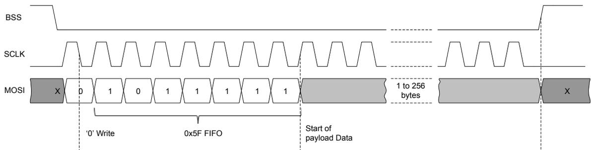
**Figure 16. SPI communication: reading bytes from FIFO**
