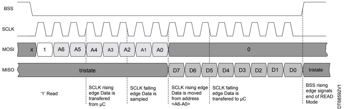
**Figure 12. SPI communication: reading of multiple bytes**
