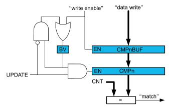
Both the TCAn.CMPn and TCAn.CMPnBUF registers are available as I/O registers, allowing the initialization and bypassing of the buffer register and the double-buffering function.
