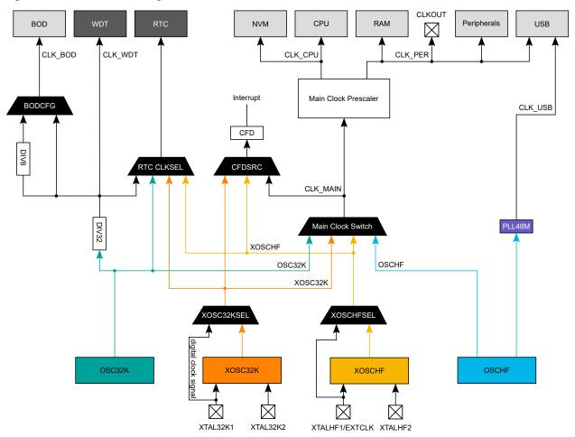
The clock system consists of the main clock and clocks derived from the main clock, as well as several asynchronous clocks:
