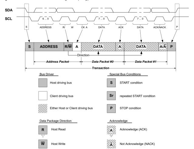
Figure 27-2. Basic TWI Transaction Diagram Topology for a 7-Bit Address Bus
