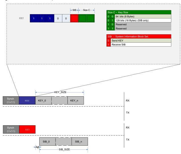
Figure 33-17 shows the transmission of a key and the reception of a SIB. In both cases, the Size C ( $SIZE\_C$ ) field in the operand determines the number of frames being sent or received. There is no response after sending a KEY to the UPDI. When requesting the SIB, data will be transmitted from the UPDI according to the current guard time setting.
