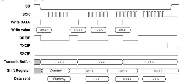
Figure 26-3. SPI Timing Diagram in Buffer Mode with BUFWR in SPIn.CTRLB Written to '0'
