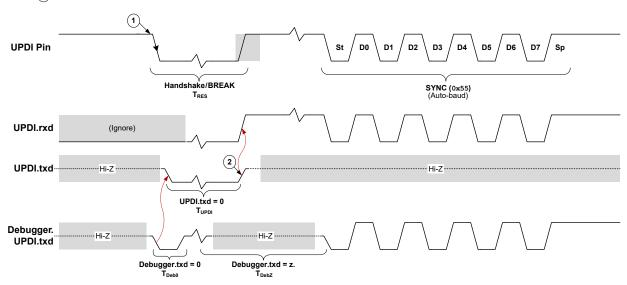
The delay given for the edge detector active drive period is a typical start-up time waiting for 256 cycles on a 32 MHz oscillator + the calibration readout. Refer to the *Electrical Characteristics* section for details on the expected start-up times.
