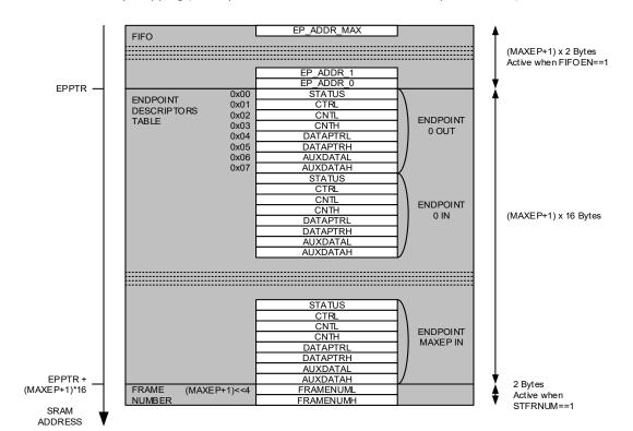
Figure 28-9. USB Memory Mapping (Descriptor table, FIFO, frame number, endpoint buffers) In RAM
