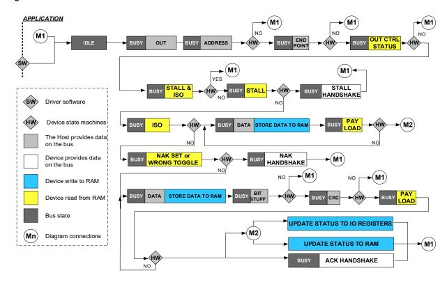
If the endpoint type matches, the USB peripheral fetches the Endpoint Data Pointer (EP[n].OUT.DATAPTR) register and waits for a DATA0 or DATA1 packet. If a PID error or any other PID than DATA0 or DATA1 is detected, the USB peripheral returns to idle and waits for the next token packet.
