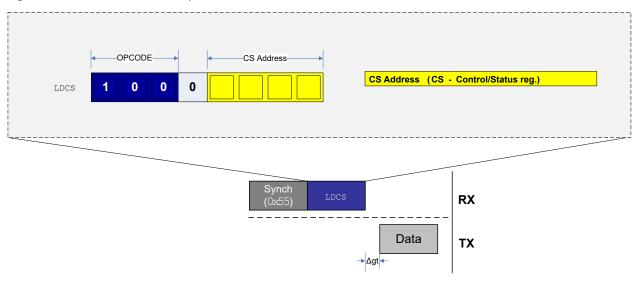
Figure 33-13 shows a typical example of LDCS data transmission. A data byte from the LDCS is transmitted from the UPDI after the guard time is completed.
