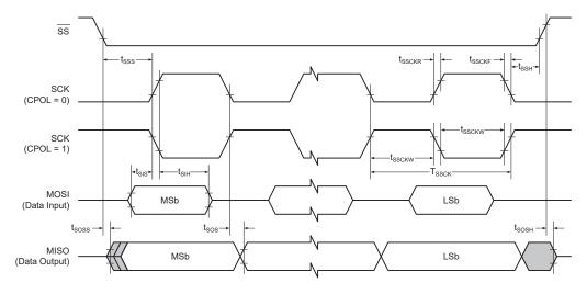
Table 37-20. SPI - Timing Characteristics in Client Mode
