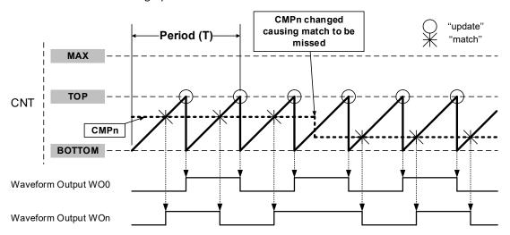
The figure below shows how changing CMPn during run-time can invert the waveform.
