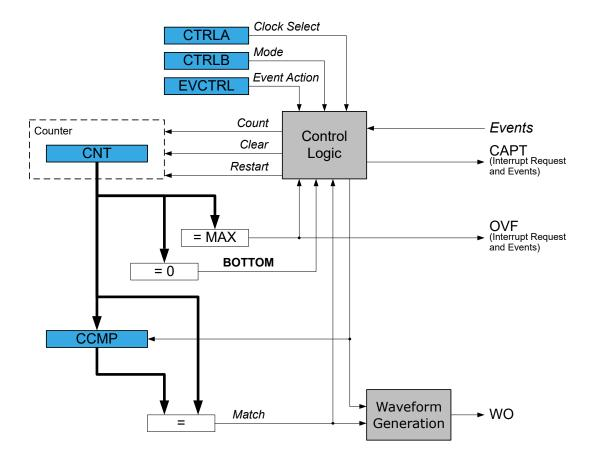
The timer/counter can be clocked from the Peripheral Clock (CLK\_PER), from a 16-bit Timer/Counter type A (CLK\_TCAn) or the Event System (EVSYS).
