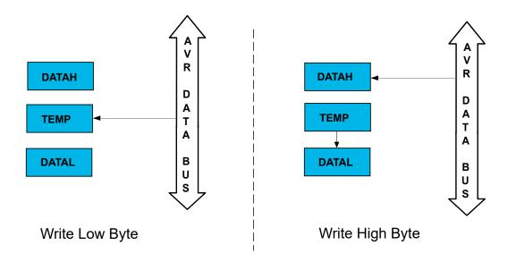
For a 16-bit write operation, the low byte register (e.g., DATAL) of the 16-bit register must be written before the high byte register (e.g., DATAH). Writing the low byte register will result in a write to the temporary register instead of the low byte register, as shown on the left side of Figure 8-2. When the high byte register of the 16-bit register is written, TEMP will be copied into the low byte of the 16-bit register in the same clock cycle, as shown on the right side of Figure 8-2.
