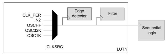
When the Clock Source (CLKSRC) bit is written to  $0 \times 1$ , LUTn-TRUTHSEL[2] is used to clock the corresponding filter and edge detector (CLK\_LUTn). The sequencer is clocked by the CLK\_LUTn of the even LUT in the pair. When CLKSRC is written to  $0 \times 1$ , LUTn-TRUTHSEL[2] is treated as OFF (low) in the TRUTH table.
