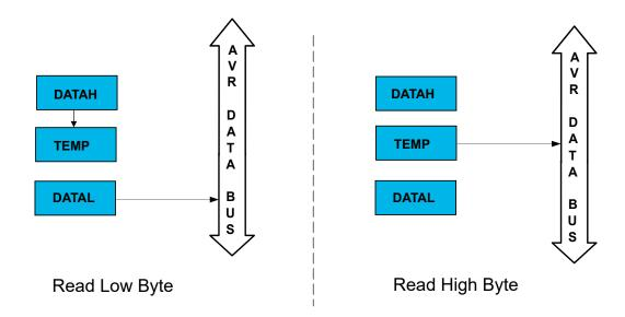
For a 16-bit read operation, the low byte register (e.g., DATAL) of the 16-bit register must be read before the high byte register (e.g., DATAH). When the low byte register is read, the high byte register of the 16-bit register is copied into the temporary register in the same clock cycle, as shown on the left side of Figure 8-3. Reading the high byte register will result in a read from TEMP instead of the high byte register, as shown on the right side of Figure 8-3.
