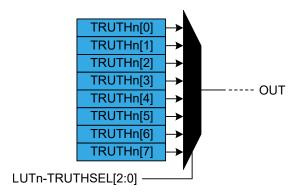
Configure the truth table inputs (LUTn-TRUTHSEL[2:0]) by writing the Input Source Selection bit fields in the LUT Control registers:
