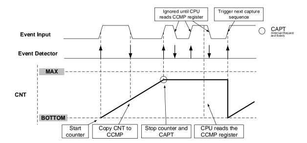
Figure 24-8. Input Capture Frequency and Pulse-Width Measurement
