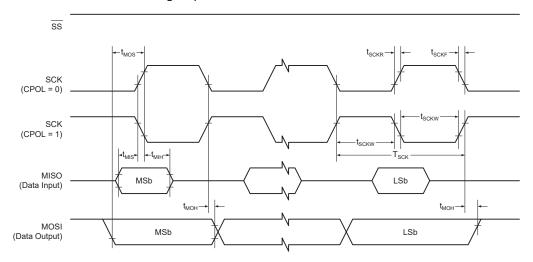
Table 37-18. USART in SPI Host Mode - Timing Characteristics
