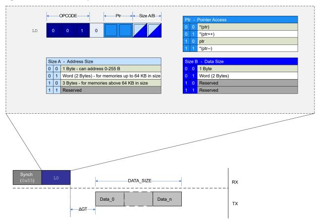
Figure 33-11 shows an example of a typical LD sequence, where the data are received after the Guard Time (GT) period. Loading data from the UPDI Pointer register follows the same transmission protocol.
