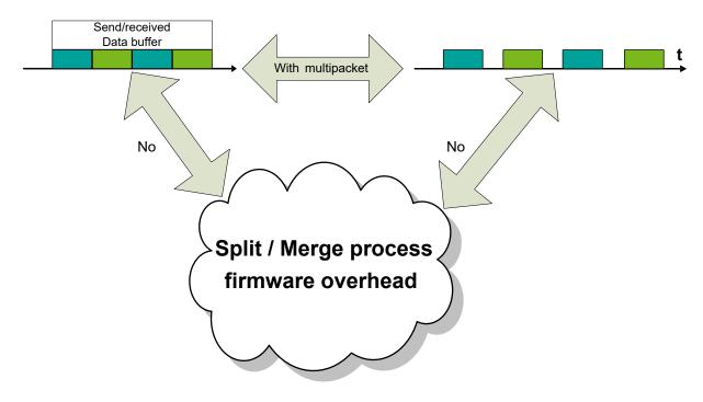
Figure 28-8. Multipacket Reduces CPU Load
