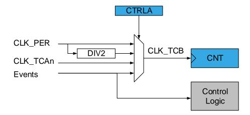
The Clock Select (CLKSEL) bit field in the Control A (TCBn.CTRLA) register selects one of the prescaler outputs directly, or an event channel as the clock (CLK\_TCB) input.
