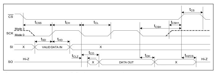
Figure 22 Synchronous data timing (mode0 and mode 3)
