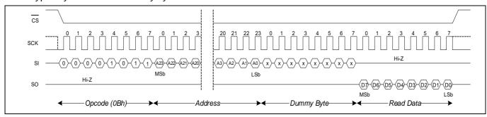
Figure 12 Fast Read Operation
