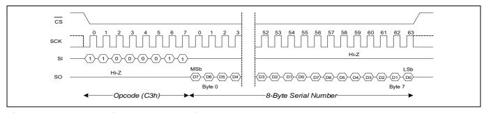
Figure 18 **Read Serial Number operation**
