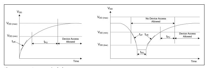
Figure 24 Power cycle timing
