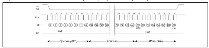
Figure 10 Memory Write (WREN not shown) Operation
