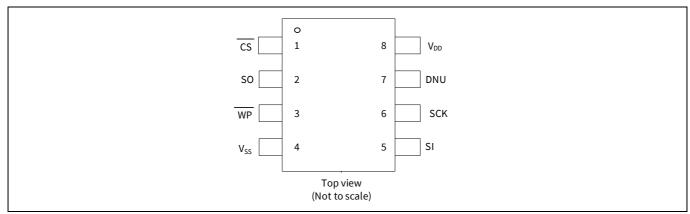
Figure 1 8-pin SOIC pinout
