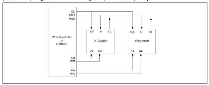
Figure 2 System configuration with SPI port
