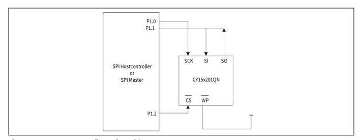
Figure 3 System configuration without SPI port
