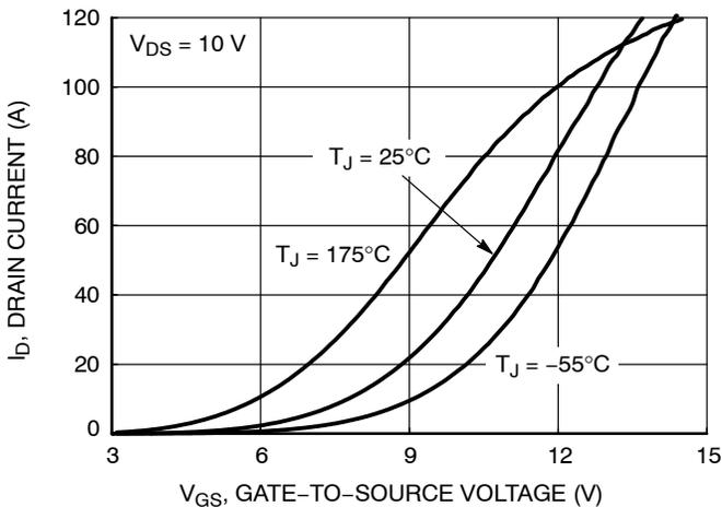
Figure 5. Transfer Characteristics
