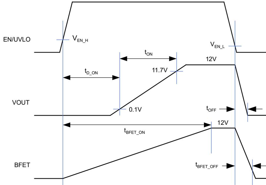
Figure 2. Turn-on Delay, Turn-on and Turn-off Time
