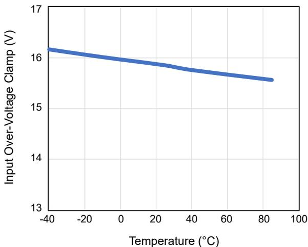
Figure 10. Input Over-Voltage Clamp vs. Temperature
