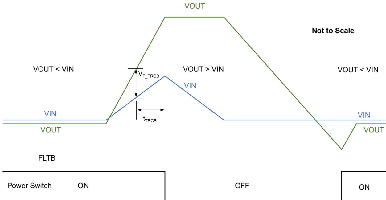
Figure 3. True Reverse Current Blocking (TRCB) Operation
