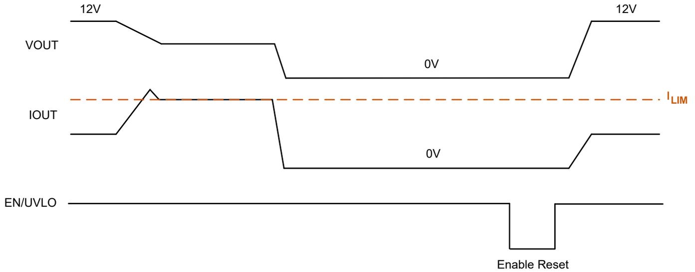
Figure 5. Current Limit Operation (AOZ18101-02 Latch-off)
