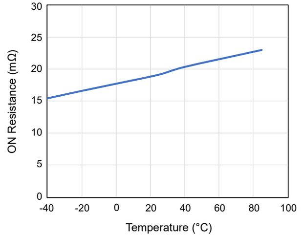
Figure 9. ON Resistance vs. Temperature (VIN = 12V)
