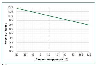
Note: Rerating depicted in this curve is in addition to the standard derating of 25% for continuous operation.
