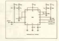
The first half of the timer is started by momentarily connecting pin 6 to ground. When it is timed out (determined by 1.1R1C1) the second half begins. Its time duration is determined by 1.1R2C2).
