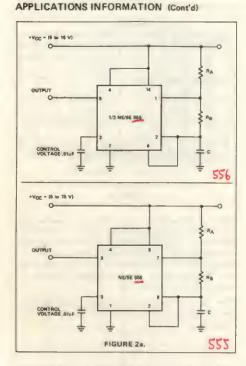
In this mode of operation, the capacitor charges and discharges between 1/3 V<sub>CC</sub> and 2/3 V<sub>CC</sub>. As in the triggered mode, the charge and discharge times, and therefore the frequency are independent of the supply voltage.
