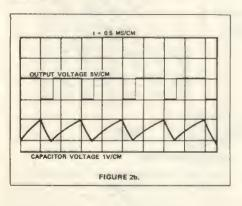
The charge time (output high) is given by:  $t_1 = 0.693 (R_A + R_B) C$ and the discharge time (output low) by:  $t_2 = 0.693 (R_B) C$ Thus the total period is given by:  $T = t_1 + t_2 = 0.693 (R_A + 2R_B) C$ The frequency of oscillation is then:  $f = \frac{1}{t_1} = \frac{1.44}{t_2}$
