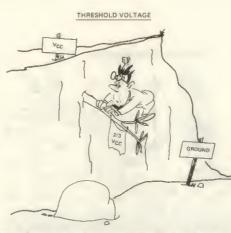
WHEN TRIGGERED, THE TIMER STARTS ITS TIMING CYCLE BY DRIVING THE OUTPUT, PIN 3, HIGH. SIMULTANEOUSLY, THE TIMING CAPACITOR STARTS CHANGING FROM ITS STEADY STATE LEVEL AT GROUND. WHEN IT REACHES 2/3 V<sub>CC</sub>, AN INTERNAL COMPARATOR IS TRIPPED, CAUSING THE CAPACITOR TO DISCHARGE TO GROUND. THIS DRIVES THE OUTPUT LOW, ENDING THE TIMING CYCLE.
