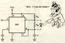
THE DUTY CYCLE IS "ON TIME" EXPRESS IN TERMS OF TOTAL CYCLE TIME, THE DUTY CYCLE IS LIMITED, UNDER NORMAL CIRCUMSTANCES, TO 50%, HOWEVER, BY ADDING A DIODE A DUTY CYCLE OF LESS THAN 50% CAN BE ACHIEVED.
