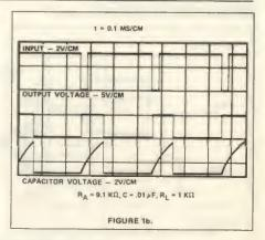
interval is independent of supply. Applying a negative pulse simultaneously to the reset terminal (pin 4) and the trigger terminal (pin 2) during the timing cycle discharges the external capacitor and causes the cycle to start over again. The timing cycle will now commence on the positive edge of the reset pulse. During the time the reset pulse is applied, the output is driven to its low state.
