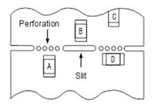
(3) Mounting components near screw holes
