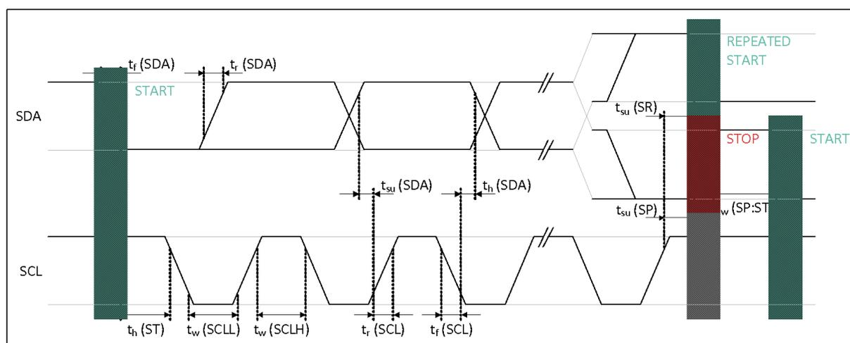
Figure 2: I<sup>2</sup>C Timing Diagram
