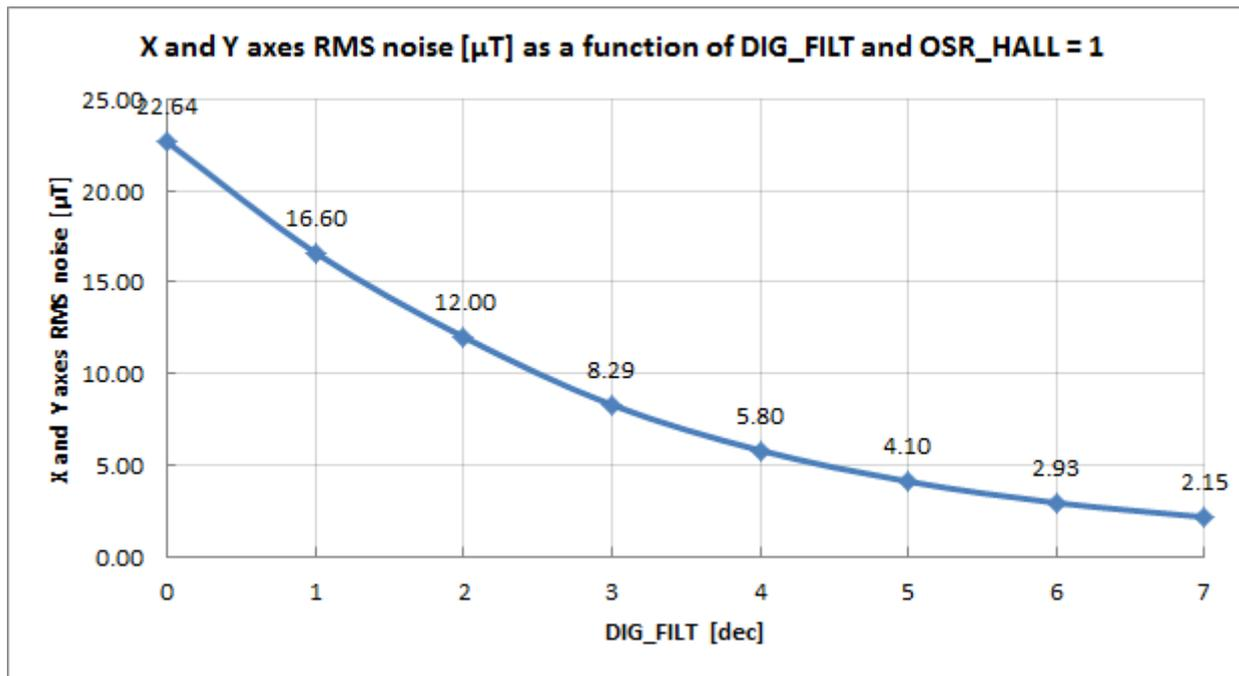
Figure 18: version 011 – XY axis RMS noise (typ)
