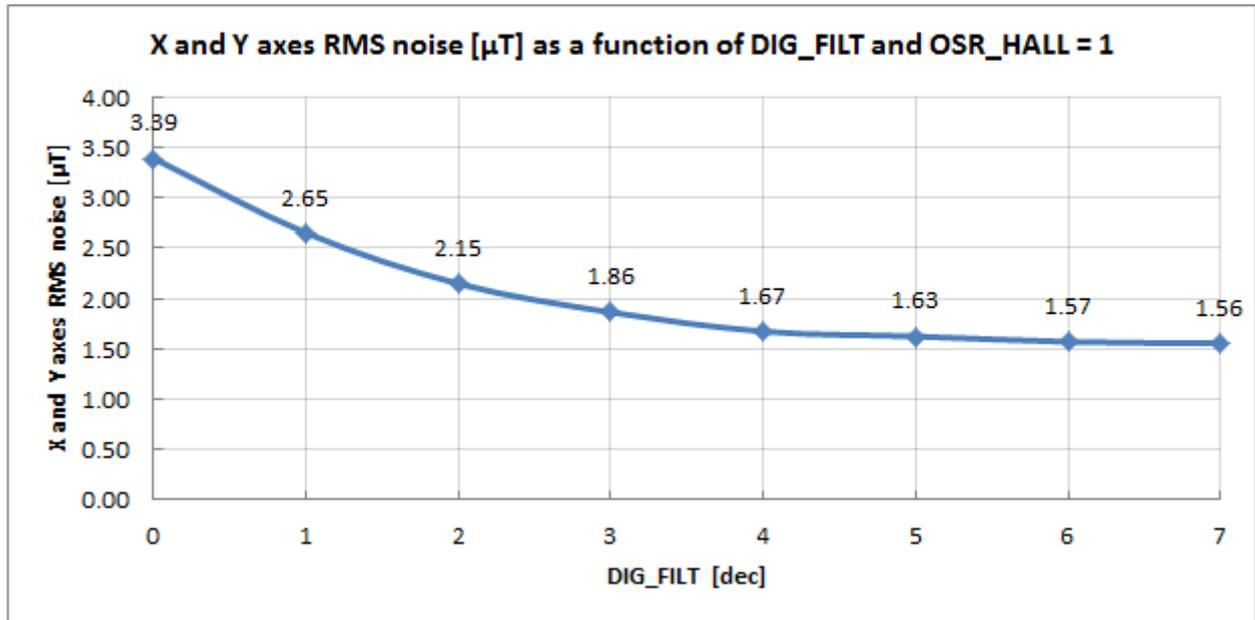
Figure 16: version 010 - XY axes RMS noise(typ)
