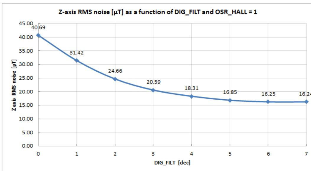
Figure 21: version 011 - Z axis RMS noise (typ)
