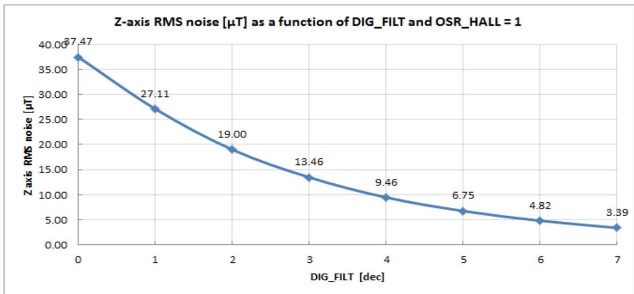
Figure 19: version 011 - Z axis RMS noise (typ)
