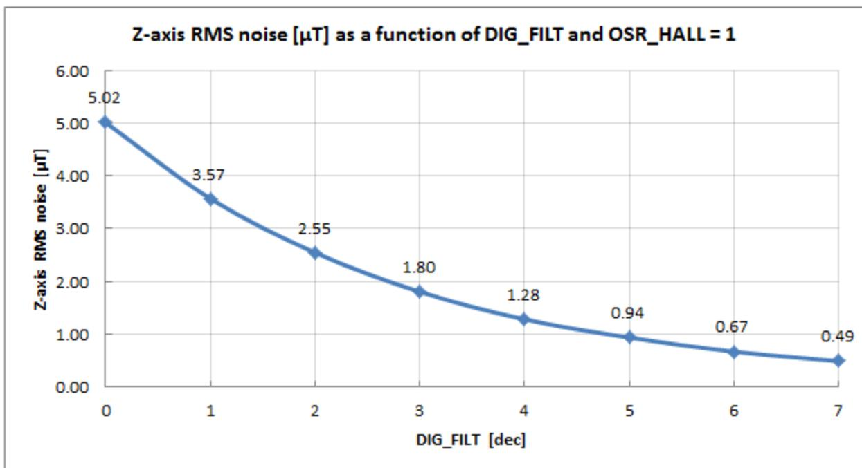
Figure 15: version 010 - Z axis RMS Noise (typ)
