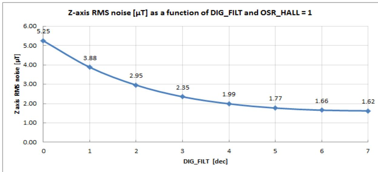
Figure 17: version 010 - Z axis RMS noise (typ)
