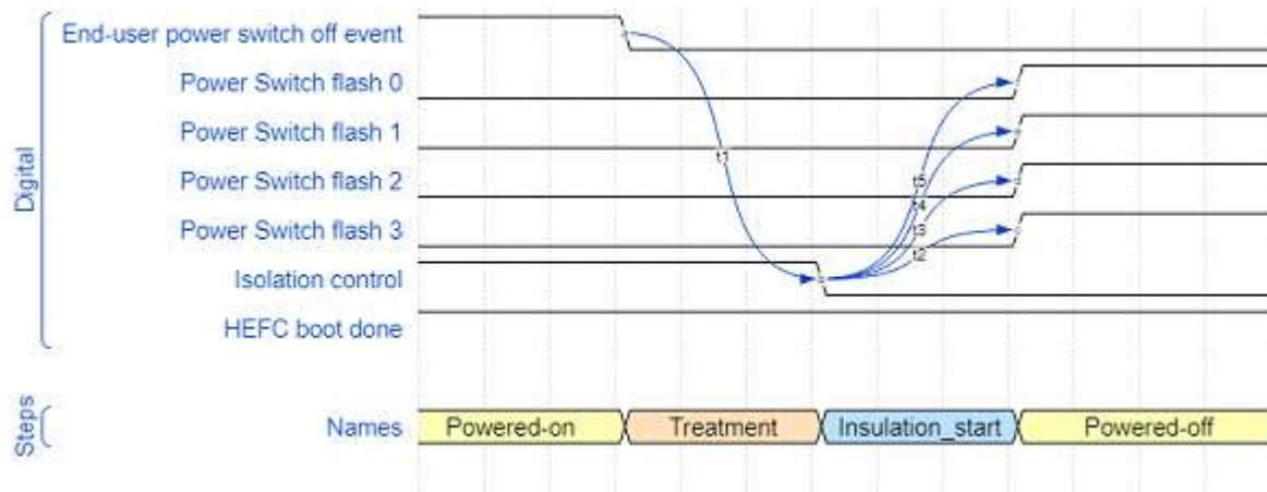
Figure 19-8. Flash Modules Power-Down Sequence – [End user]
