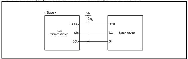
Remark 1. R<sub>b</sub>[Ω]: Communication line (SOp) pull-up resistance, C<sub>b</sub>[F]: Communication line (SOp) load capacitance, V<sub>b</sub>[V]: Communication line voltage
