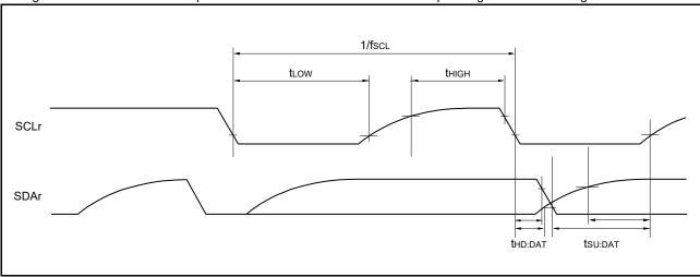
Remark 1.  $R_b[\Omega]$ : Communication line (SDAr, SCLr) pull-up resistance,  $C_b[F]$ : Communication line (SDAr, SCLr) load capacitance,  $V_b[V]$ : Communication line voltage
