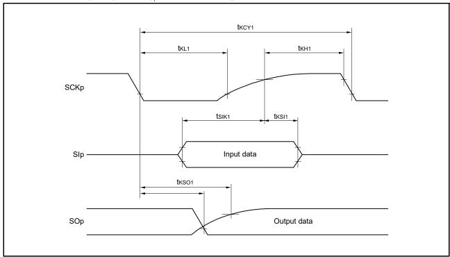
Timing of serial transfer in the SPI (CSI) communications in the master mode with devices operating at different voltage levels when DAPmn = 0 and CKPmn = 1, or DAPmn = 1 and CKPmn = 0
