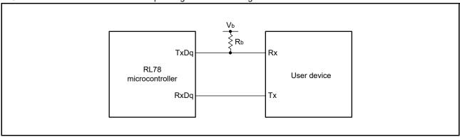
Bit width in the UART communications with devices operating at different voltage levels (reference)
