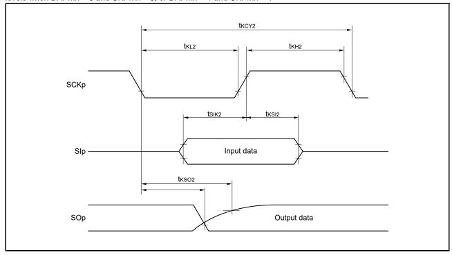
Timing of serial transfer in the SPI (CSI) communications in the slave mode with devices operating at different voltage levels when DAPmn = 0 and CKPmn = 1, or DAPmn = 1 and CKPmn = 0
