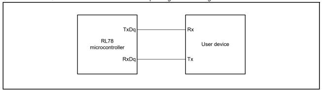
Bit width in the UART communications when interfacing devices operate at the same voltage level (reference)
