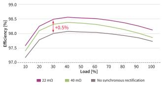
CoolMOS™ S7 brings more efficiency to power supplies when used in an active rectification bridge.
