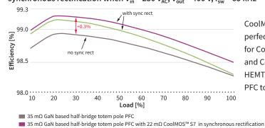
35 mΩ GaN based half-bridge totem pole PFC with 40 mΩ CoolMOS™ S7 in synchronous rectification
