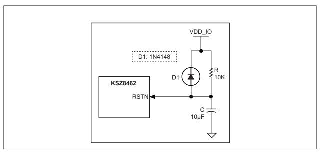
The following reset circuit is recommended for applications where reset is driven by another device (e.g., CPU or FPGA). At POR, R, C, and D1 provide the necessary ramp rise time to reset the KSZ8462 device. The RST\_OUT\_N from CPU/FPGA provides the warm reset after power-up.
