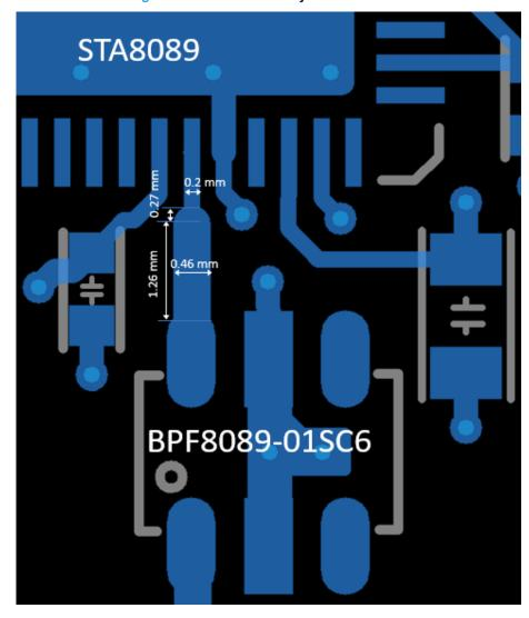
Figure 6. Recommended layout for STA8089
