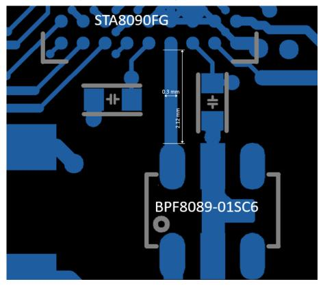
Figure 7. Recommended layout for STA8089FG
