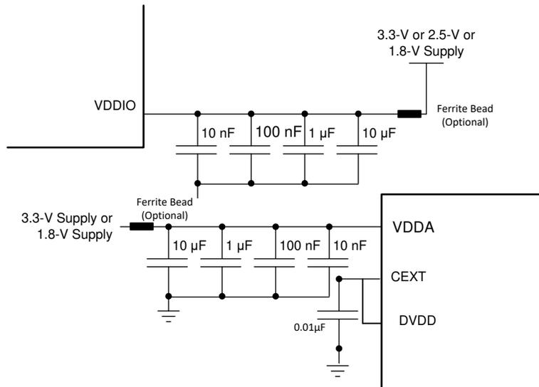
**Figure 9-1. DP83TD510E Single Power Supply Decoupling Recommendation**
