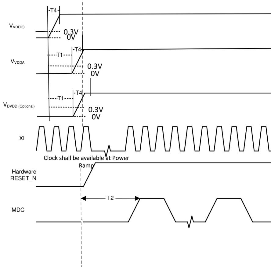
**Figure 6-1. Power-Up Timing**
