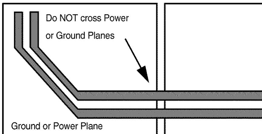
**Figure 10-2. Differential Signal Pair and Plane Crossing**
