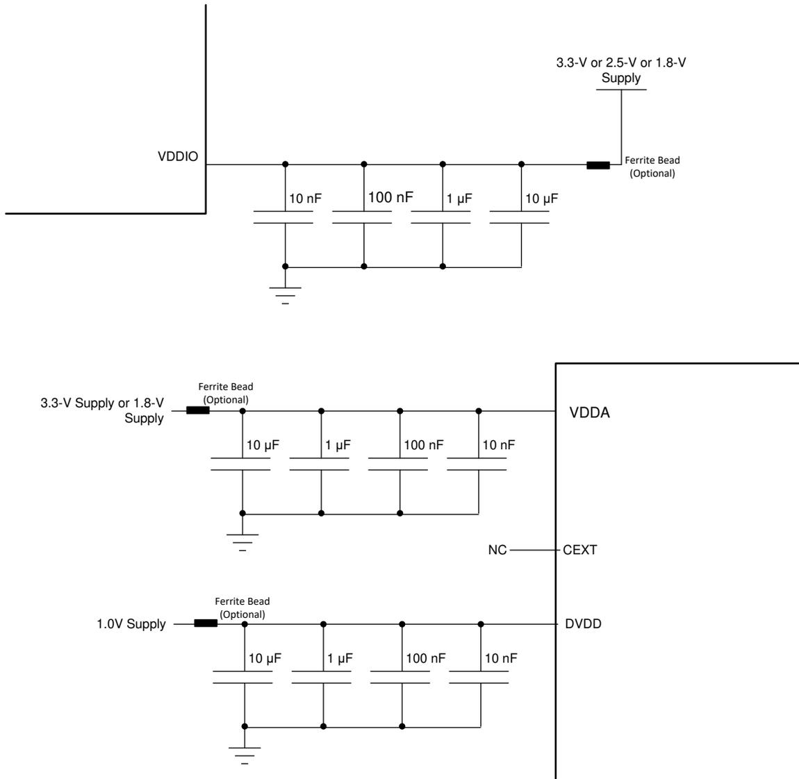
Figure 9-2. DP83TD510E Dual Supply Power Supply Decoupling Recommendation
