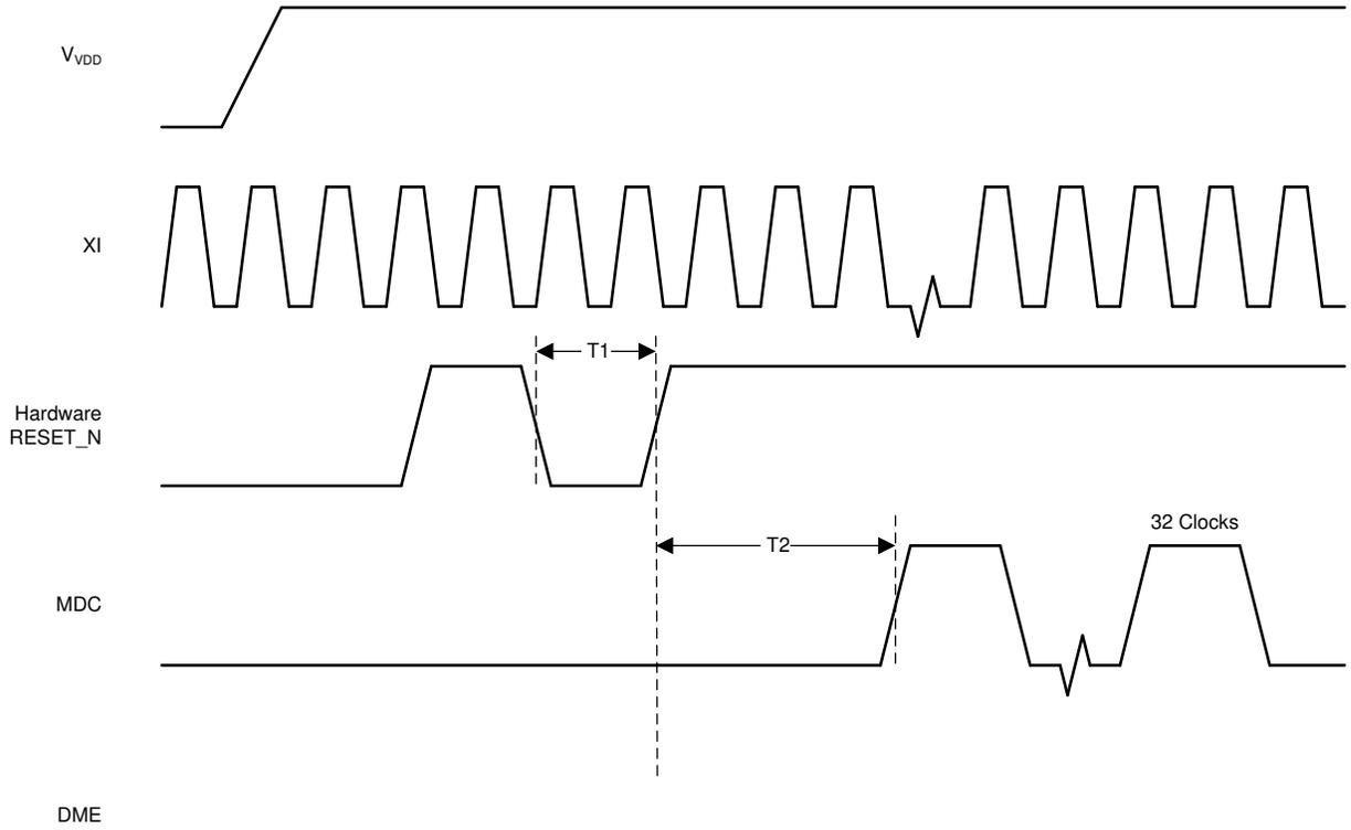
**Figure 6-2. Reset Timing**
