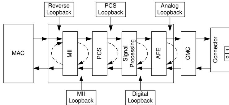
Figure 7-5. Loopback Test Modes
