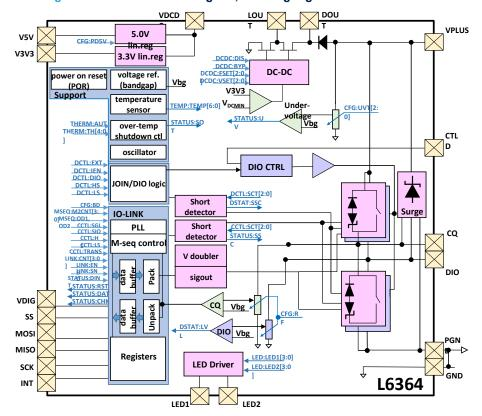
Figure 19. Detailed block diagram, showing register field connections
