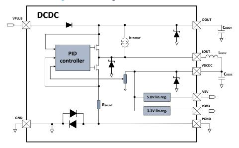
Figure 11. Block diagram of DC-DC converter
