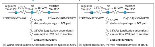
Figure 15. Example of thermal power dissipation estimation
