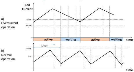
Figure 13. Overcurrent operation
