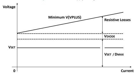
Figure 12. Minimum supply voltage
