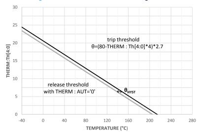
Figure 9. L6364 thermal shutdown configuration
