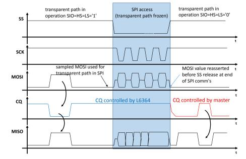
Figure 7. Illustration of operation in transparent mode
