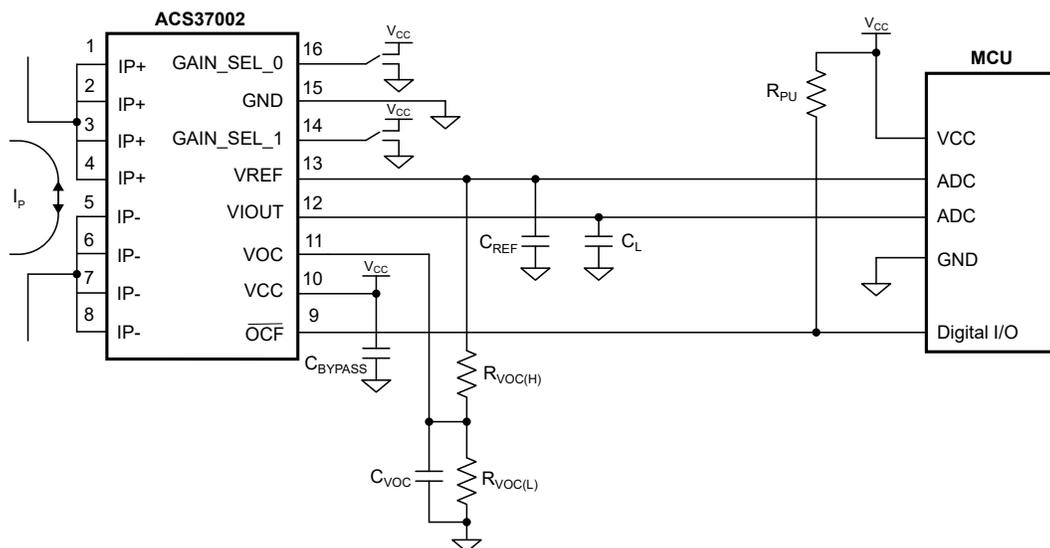
**Figure 1: Typical Bidirectional Application.**
