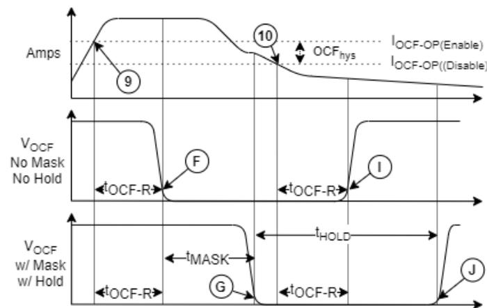
**Figure 15: General Fault Timing.**
