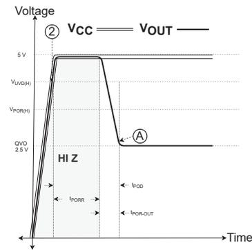
Figure 5:  $t_{POD}$  behavior UVD disabled,  $R_L$  = Pull-Up
