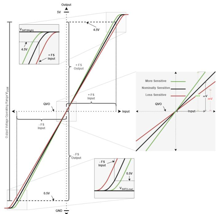
Figure 10:  $V_{OOR}$ ,  $V_{SAT}$  and SENS with Full Scale
