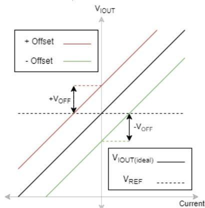
Figure 9: Offset ( $V_{OFF}$ ) Between  $V_{IOUT}$  and  $V_{REF}$
