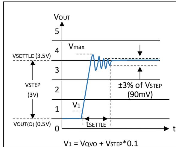
Figure 19: Overshoot and Settling Time (3 V step shown)
