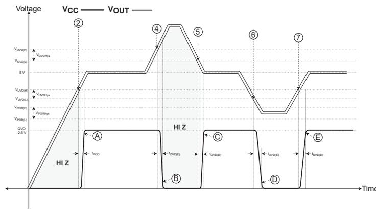
Figure 8:  $t_{POD}$ ,  $t_{OVD(E/D)}$ , and  $t_{UVD(E/D)}$  with  $R_L = \text{Pull-Up}$
