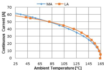
**Figure 24: Maximum Continuous Current at a Given  $T_A$**
