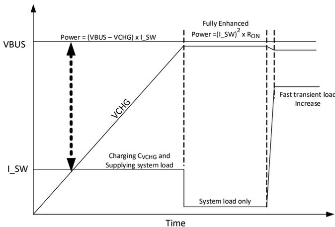
Figure 24. Soft start power dissipation
