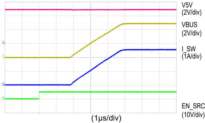
Figure 14. Source Mode Start Up by Enable
