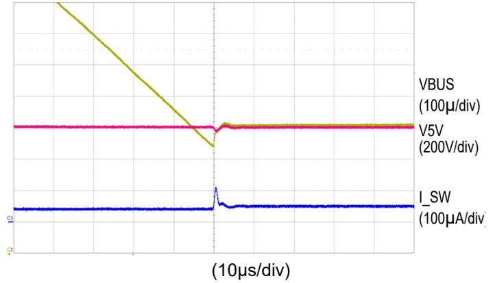
Figure 21. Source Mode Recovery from True Reverse Current Blocking Release
