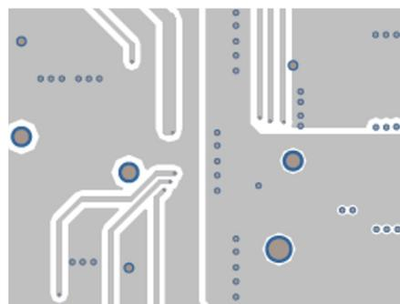
Figure 30. Bottom layer layout. Create a large electrically isolated thermal pad.
