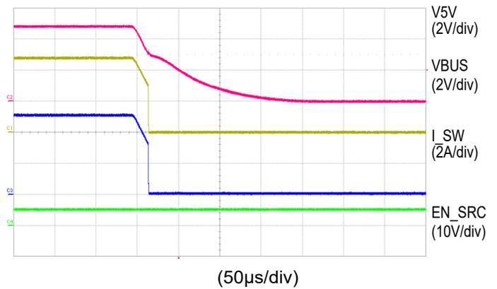
Figure 17. Source Mode Shut Down by V5V Ramp
