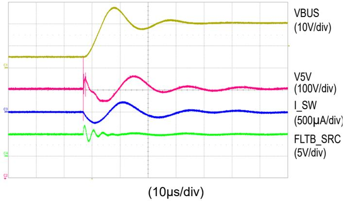
Figure 20. Source Mode True Reverse Current Blocking
