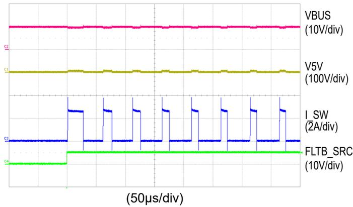
Figure 22. Source Mode Start Up to Short Condition
