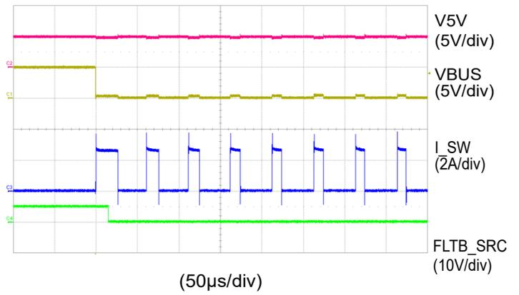
Figure 19. Source Mode Short Circuit Protection, Thermal Shut Down, and Auto Restart
