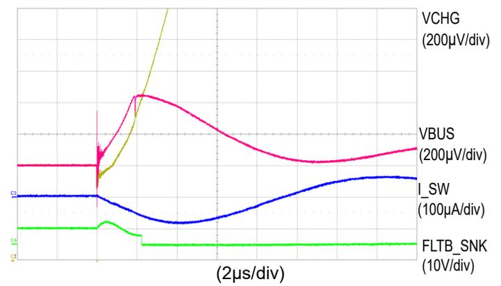
Figure 13. Sink Mode True Reverse Current Blocking (VBUS=5V)
