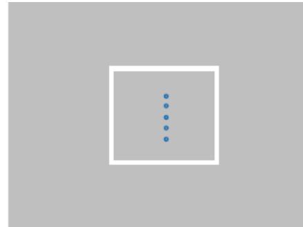
Figure 28. Inner layer layout. Create electrically isolated thermal island with flooded plane.
