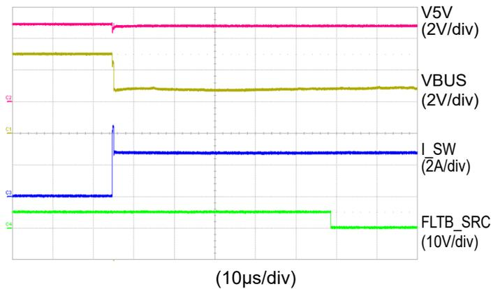
Figure 18. Source Mode Over Current Protection (Load = 1.2Ω)
