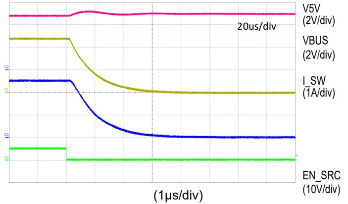
Figure 15. Source Mode Shut Down by Disable
