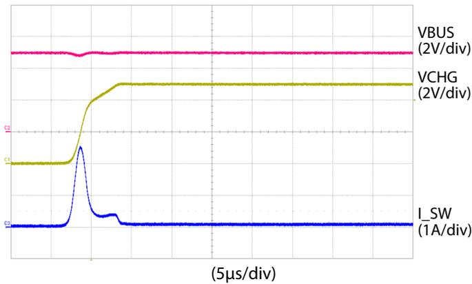
Figure 10. Sink Mode Soft Start Ramp (VBUS = 5V)
