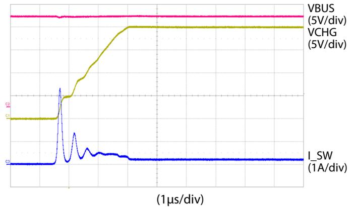
Figure 11. Sink Mode Soft Start Ramp (VBUS = 20V)
