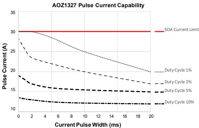
Figure 26. Pulsed current magnitude vs duration for a given duty cycle
