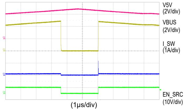
Figure 23. Source Mode Over Voltage Protection
