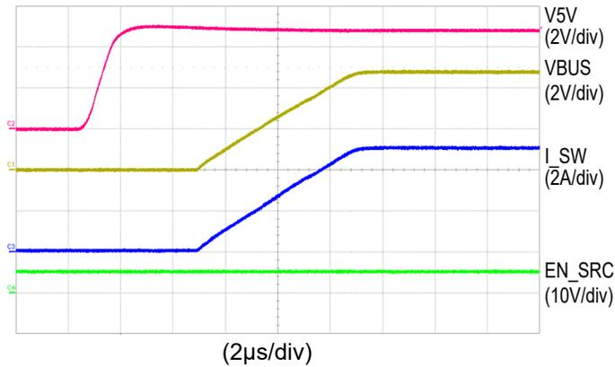
Figure 16. Source Mode Start Up by V5V Ramp
