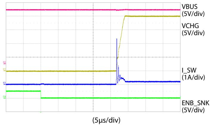
Figure 9. Sink Mode Soft Start Ramp (VBUS = 20V)
