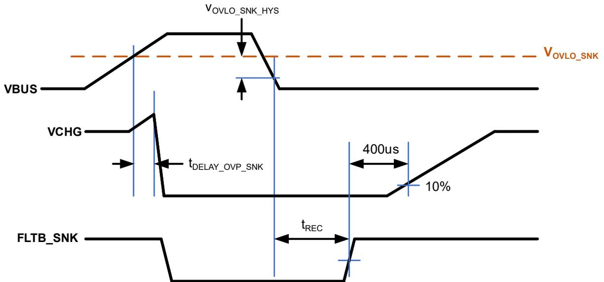
Figure 4. Over-Voltage Protection (OVP) Operation in Sink Mode
