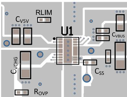
Figure 27. Top layer layout. Maximum number of VIAs from top layer exposed pad to inner layer.
