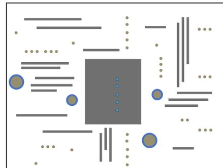
Figure 29. Inner layer layout. Create an isolated island with no flooded plane.
