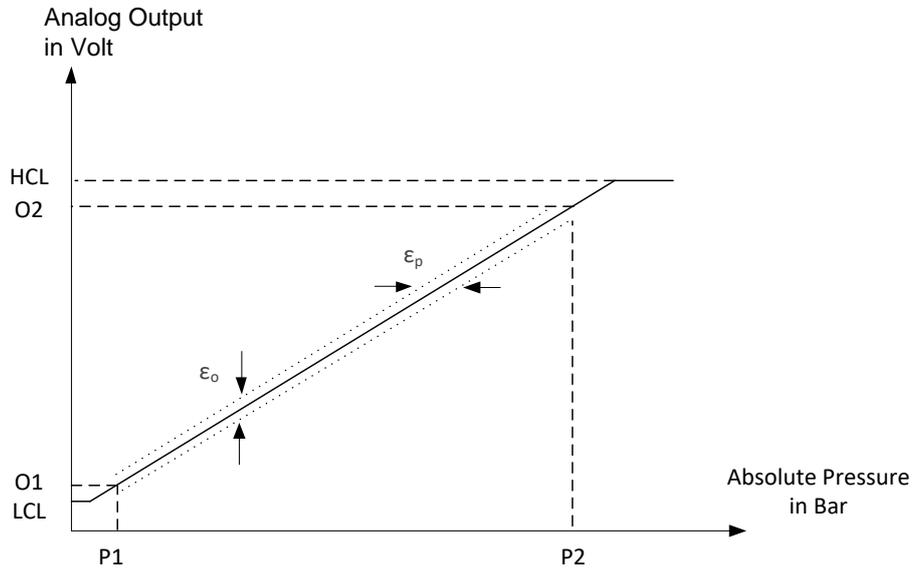
Figure 5: Pressure transfer function description at room temperature
