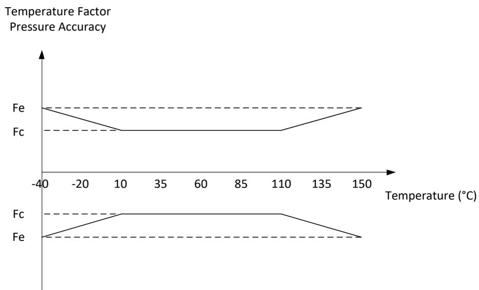
Figure 6: Pressure accuracy temperature factor
